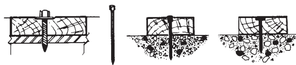
Figure 40-3: Types of Pins
