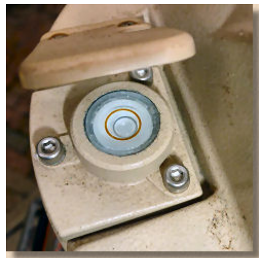
Centering the level-bubble on an automatic level
